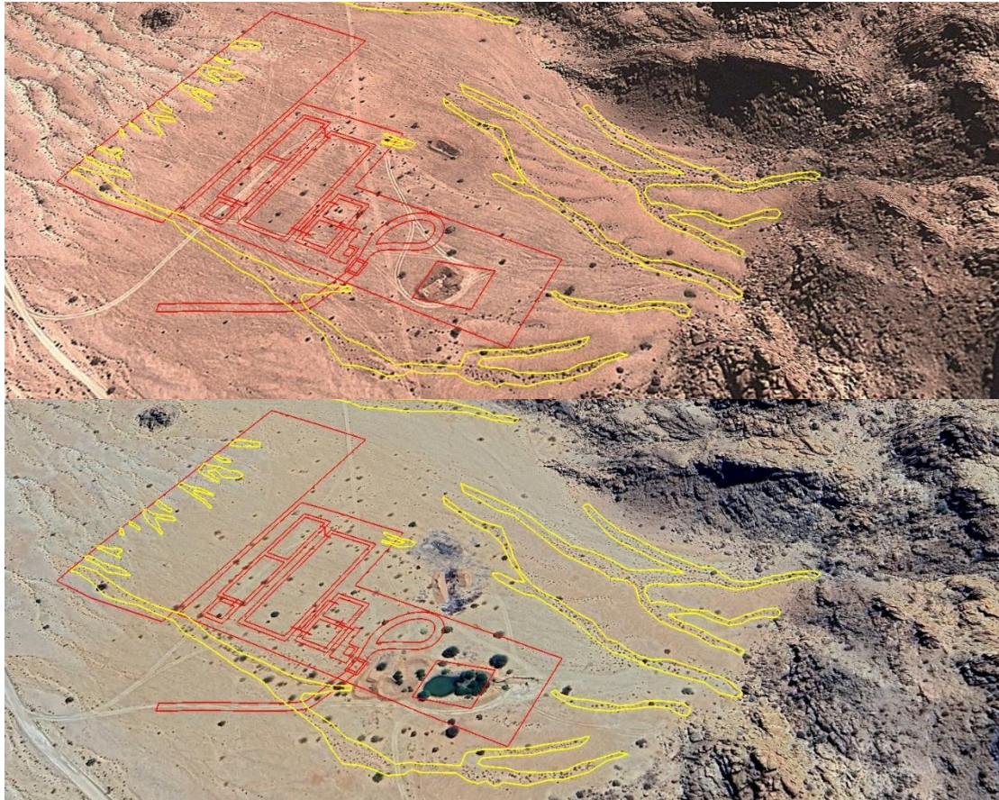
Figure 7: View of the affected drainage line network, indicating how the system and surroundings, which previously had been natural (Top - Google Earth 2010), have become quite degraded and modified since the establishment of the waste disposal site, which has also encroached into two of these drainage lines (Bottom – Google Earth 2023).
