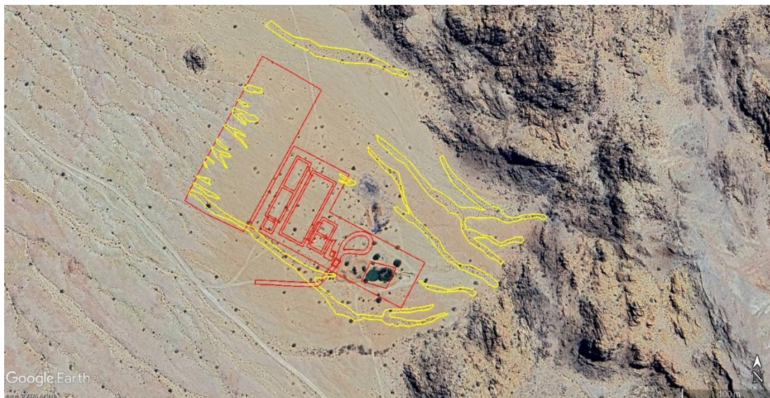
Figure 5: Recent aerial images (Google Earth 2023) indicate the existing waste disposal site (landfill and sewage disposal), which contributes to the modification of at least one of the drainage lines in the area. The proposed WWTW and irrigation area (red), may also have an impact on some of these drainage lines (yellow).
