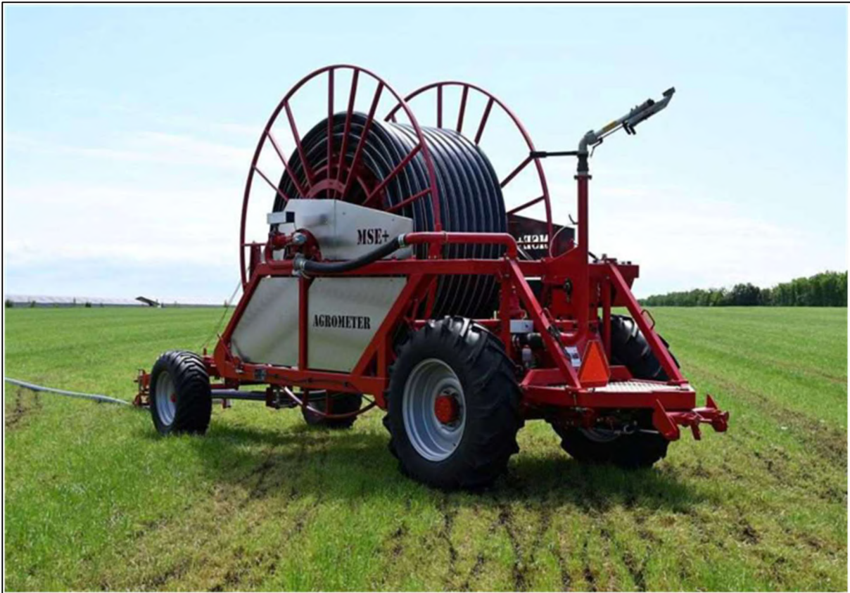
Figure 6: Example of a self-propelled crawling irrigator which may be utilised.
