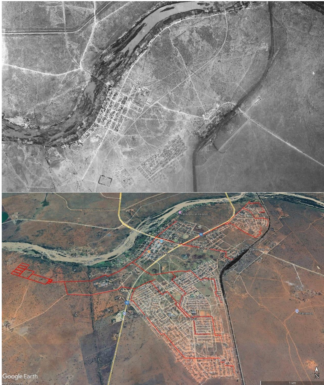
Figure 4: Aerial view of the WWTW and sewer network area. Historically (Top – National Geospatial Database 1956), the Vaal River remains prominent, though current artificial wetlands are completely absent (Bottom – Google Earth 2023), confirming that they are a consequence of the urban expansion over time.
