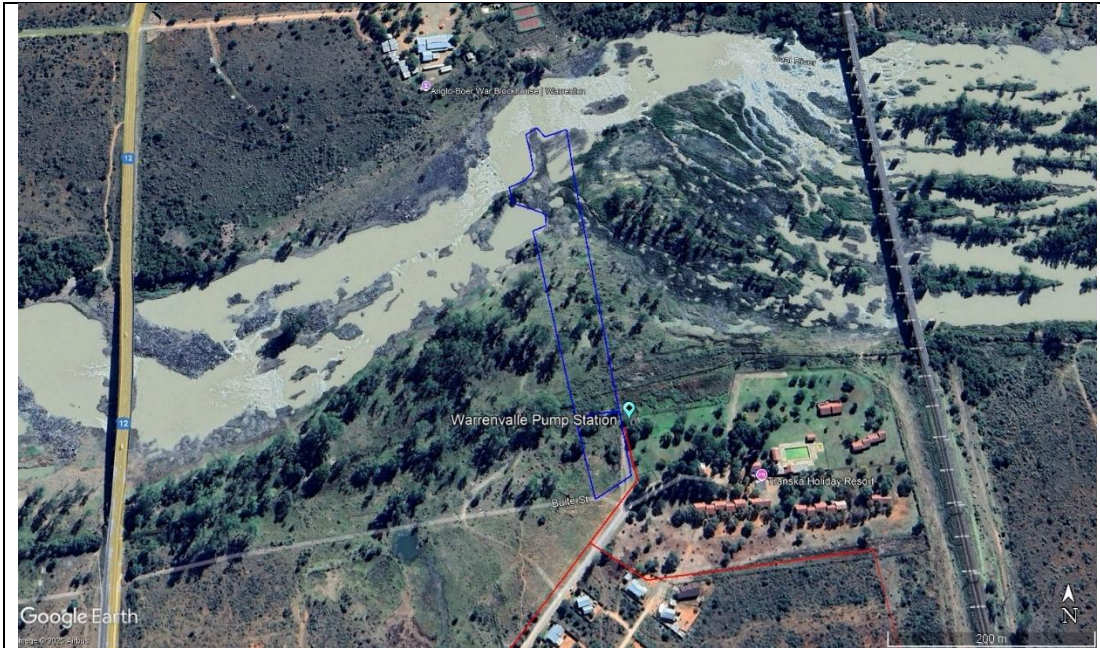
View of the Vaal River, its floodplain and riparian zone (blue), which indicates extensive wetland areas. The proposed sewer network (red) and warrenvale pump station are indicated, which will clearly encroach into the floodplain of the river.
