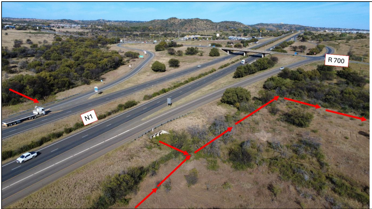
Figure 2: Proposed pipeline crossing of the N1.
