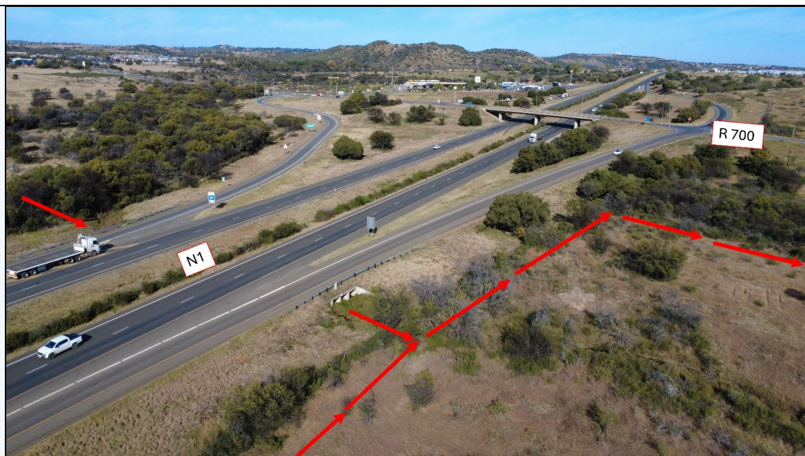
Figure 4: Proposed pipeline crossing of the N1.
